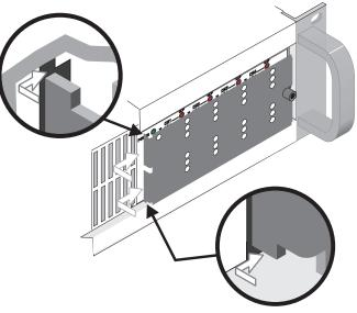
**4.** Make sure the LED's are visible, then tighten the screw with the hex key. Do not over tighten!
